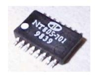
Operating Temperature: -25°C to +55°C. Storage Temperature: -55°C to +80°C.
